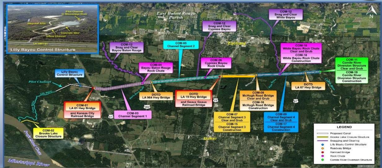
**USACE will deliver 20 construction contracts**, to include four main channel segments, two vehicular bridges, one railroad bridge, three rock chutes, diversion structure, and four low flow pumping stations.
